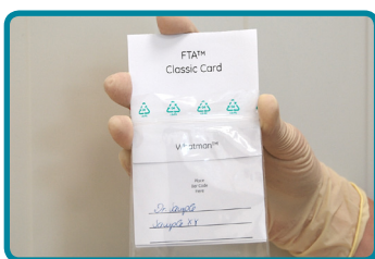
Put FTA® Card in a protection clip bag
