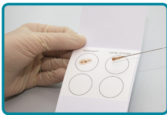
Press Sample onto FTA® Card
